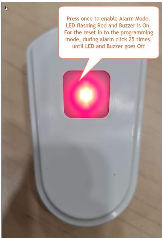
When Programming mode is activated, Panic Button goes to the Access Point Mode, and using any Wi-Fi enabled device, i.e., Laptop, Tablet or Smart Phone you can connect directly to the web interface of the Panic Button.
