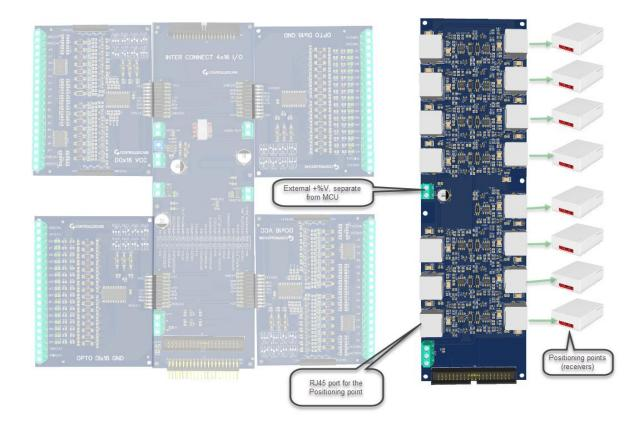
Distance between position points and dedicated port is limited to 750 meters. If to use CAT6 cable, then cable run can be longer, but not more than 1200 meters.
