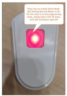
When Programming mode is activated, Panic Button goes to the Access Point Mode, and using any Wi-Fi enabled device, i.e., Laptop, Tablet or Smart Phone you can connect directly to the web interface of the Panic Button.
